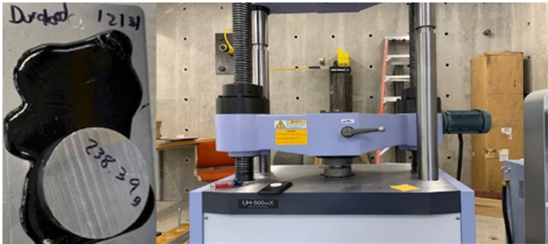
Figure 6. Sample, Cylindrical Steel Bar, Low Frame Shimadzu Universal Testing Machine
