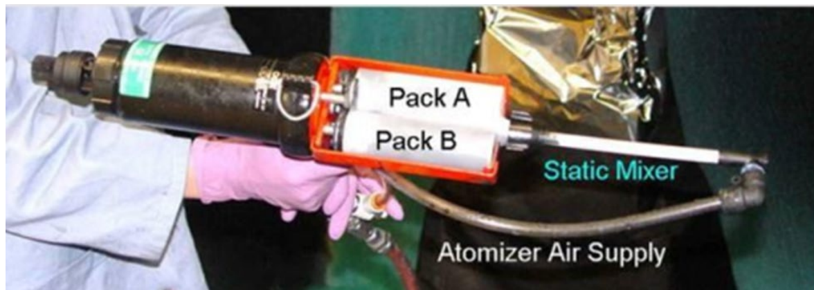
Figure 4. Portable Plural Component System for Spray Application of Polyurea Samples
