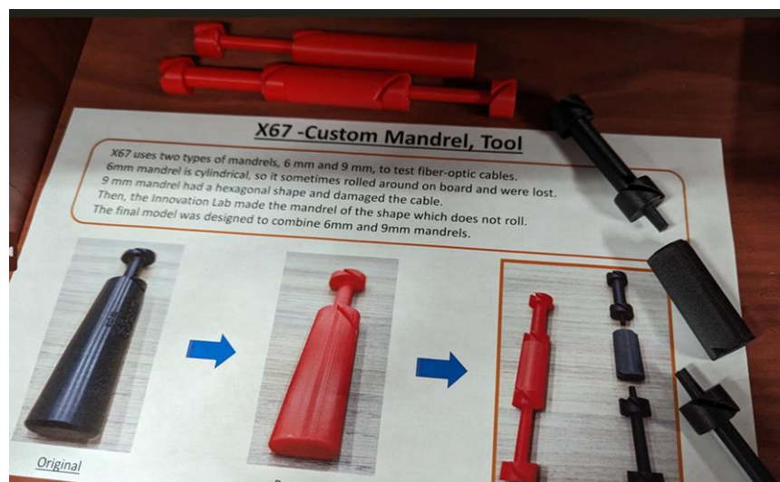
Figure 27. Custom Mandrel Tool Improved performance and consolidated two tools into one.
