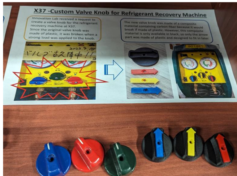
Figure 26. Custom Valve Knob Replaced the easily broken original plastic version with a carbon fiber reinforced plastic.
