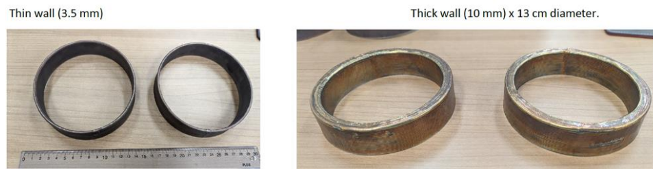
Figure 29. Meltio DED Pipe Test Unit Samples – Material SUS308L
