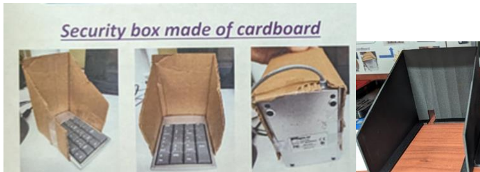
Figure 25. Security Box for Numeric Keypad Replaced makeshift cardboard box.
