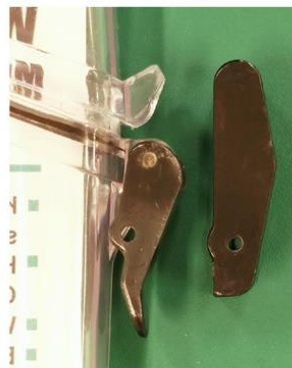
Figure 7. Case Study #3 – Card Holder Hinge Replacement Part
