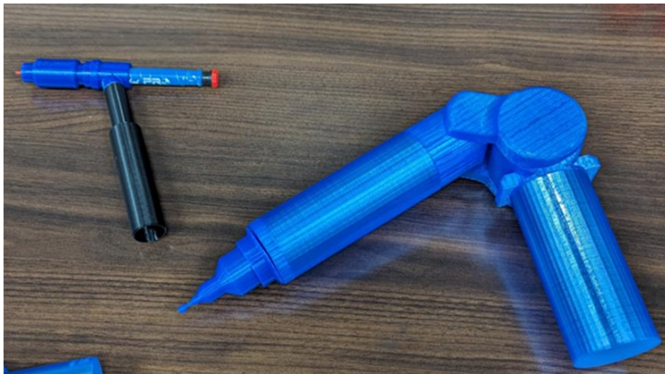
Figure 23. (Left) Welding Handset with Pen Mount for Practicing Welding Techniques; (Right) Faro 3D Scanner Replica End Arm Effector
