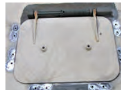
HIMARS repair – composite armor
