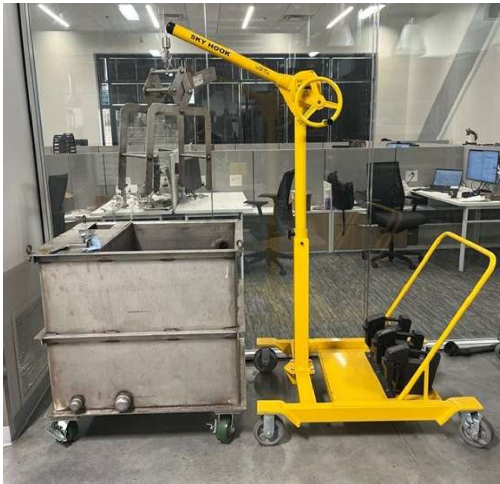
Figure 2. Build Plate Transfer Using Sky Crane and Gripper Assembly
