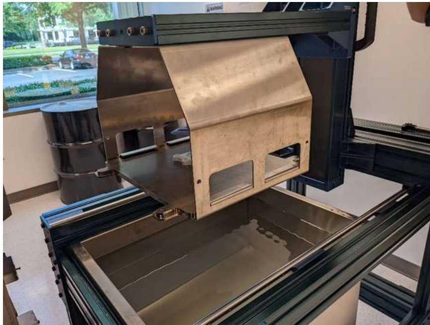
Figure 3. Stationary Build Plate Transfer System for Navy
