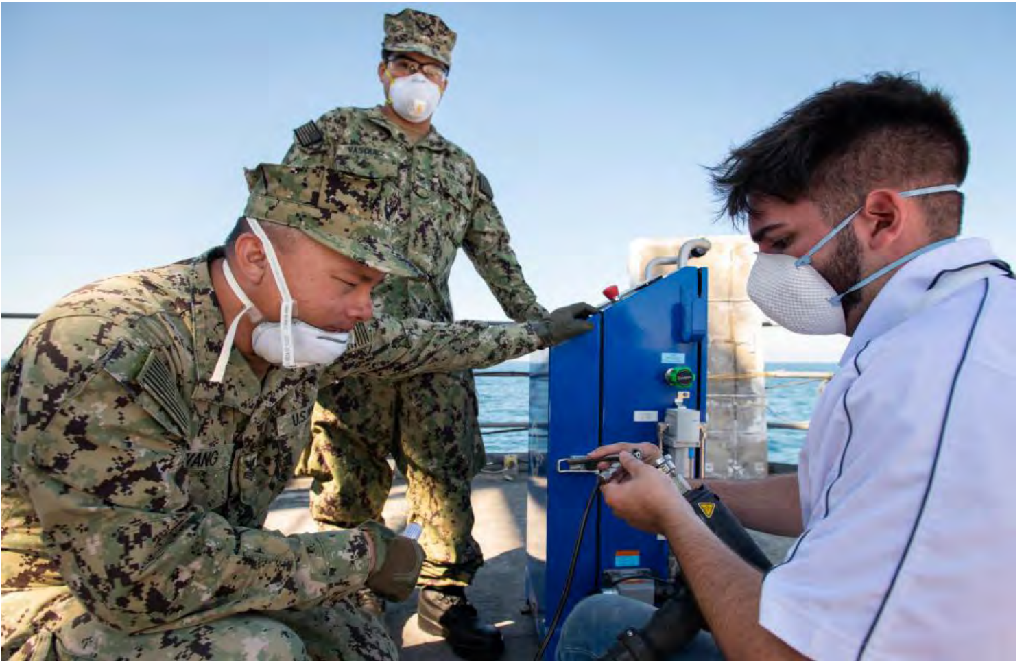
Two hull maintenance technicians of the Navy's Surge Maintenance program listen as EWI Cold Spray Research Engineer Sam Bedard briefs them on the use of the Centerline SST low-pressure cold spray system aboard the Self Defense Test Ship while underway off the coast of Naval Surface Warfare Center, Port Hueneme Division, during the 2022 REPTX. (US Navy photo by Eric Parsons.)
