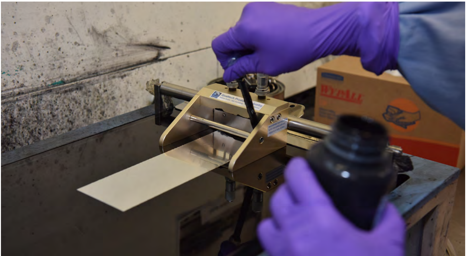
A PPG scientist coats out NMP-free cathode slurry onto aluminum foil. These films are then cured and calender-pressed to create a cathode before electrochemical testing. (Photo courtesy of PPG Industries, Inc.)
