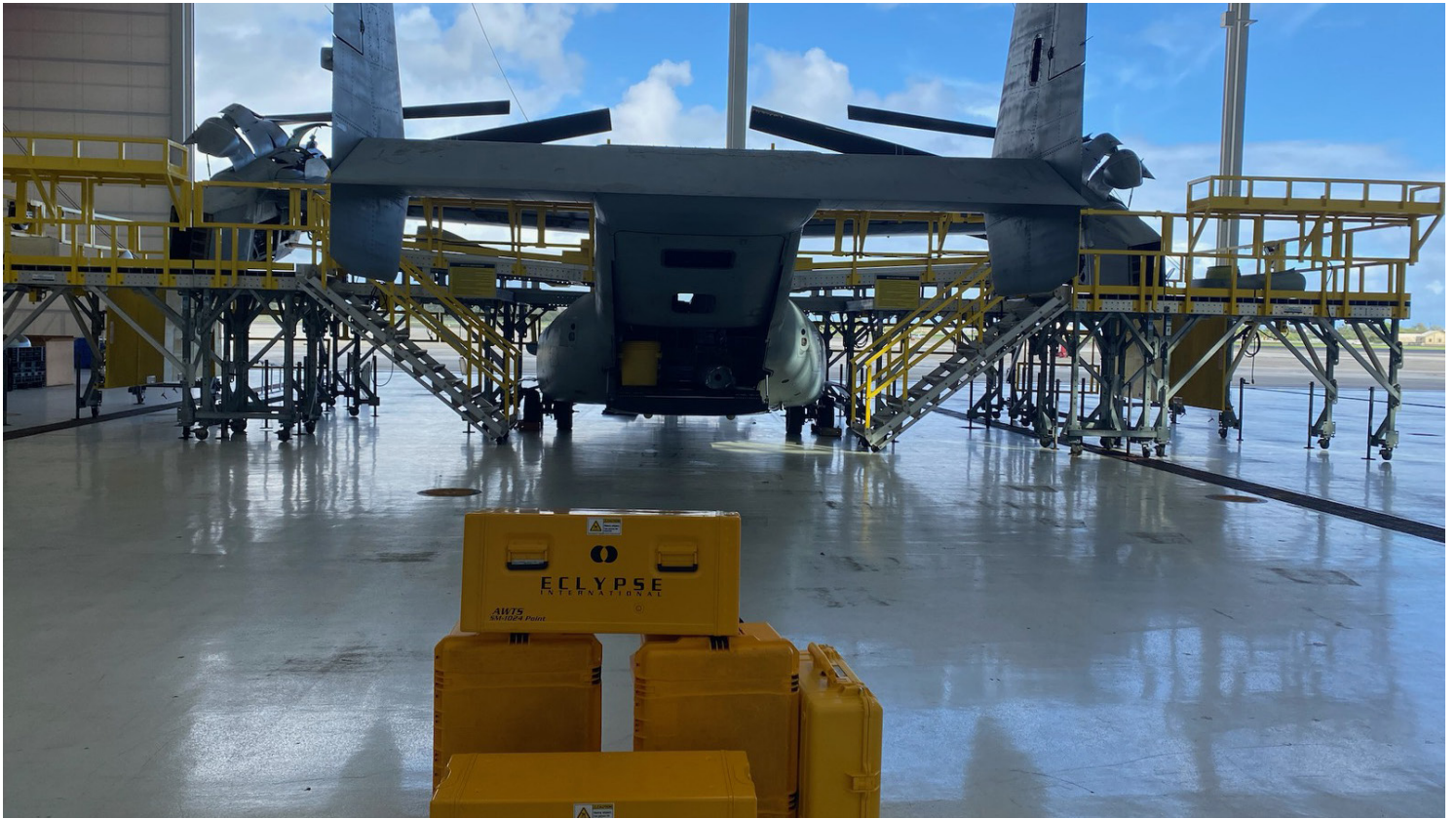
A maintenance crew prepares to test the wiring on a V-22 Osprey. (Photo courtesy of Eclipse International.)
