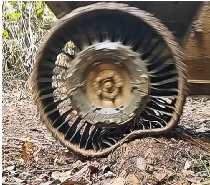
The Tweel airless tire deflects upon impact during testing at the US Army Tropic Regions Test Center (TRTC) in Suriname. (Photo by Carlos Mora.)
