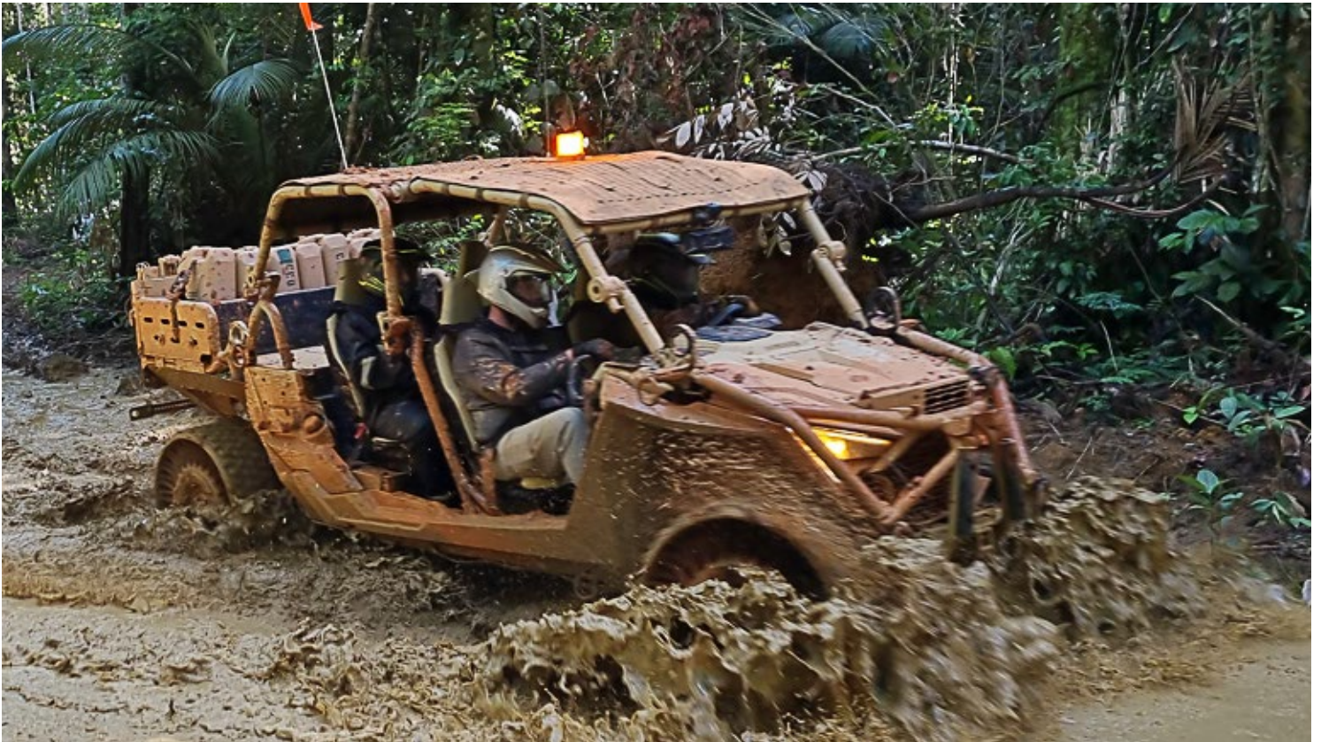
The Airless Tire project team conducts testing while driving through interior jungle trails located at the US Army Tropic Regions Test Center (TRTC) in Suriname. (Photo by Carlos Mora.)
