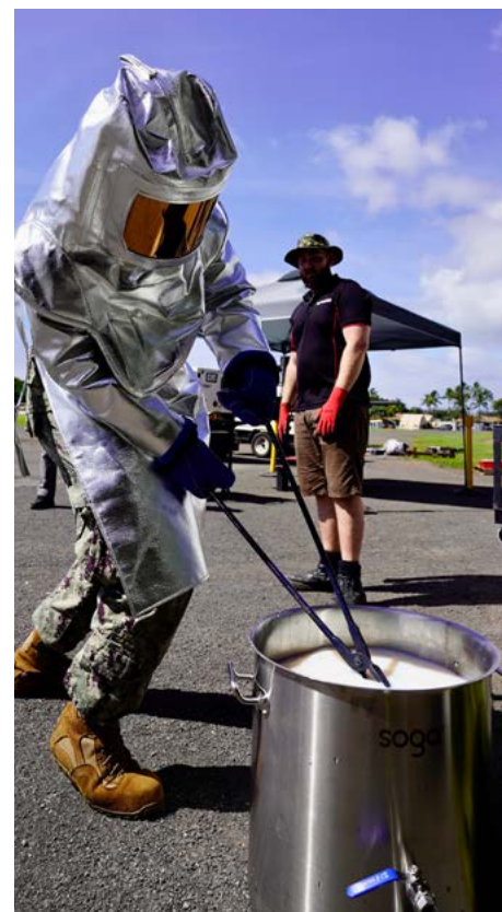
A Naval Postgraduate School student quenches a cold spray part to repair a cooler head near PHNSY during the REPTX Salv-Ex event in May. (US Navy photo by Claudia LaMantia.)
