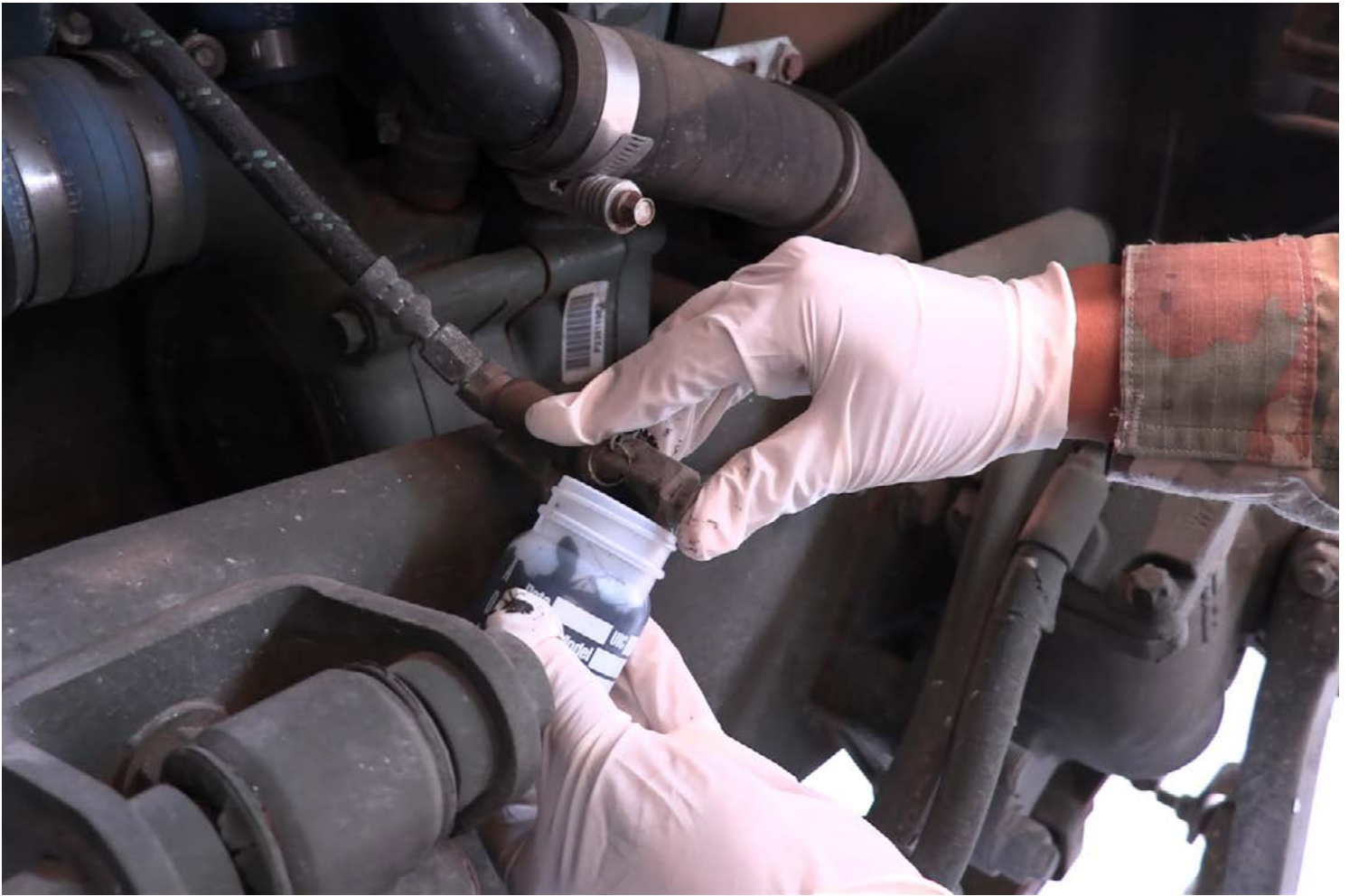
A wheeled vehicle mechanic at the 39th Transportation Battalion takes an oil sample from a 915A5 Line Haul Tractor Truck at the unit's headquarters on Kleber Kaserne in Kaiserslautern, Germany. (US Army photo by Sgt. 1st Class John Freese.)
