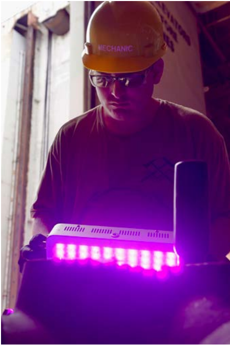
A Sailor uses UV light to solidify a sun resolution patch aboard the USS Tarawa during the REPTX Salv-Ex event in May at PHNSY. (US Navy photo by Claudia LaMantia.)
