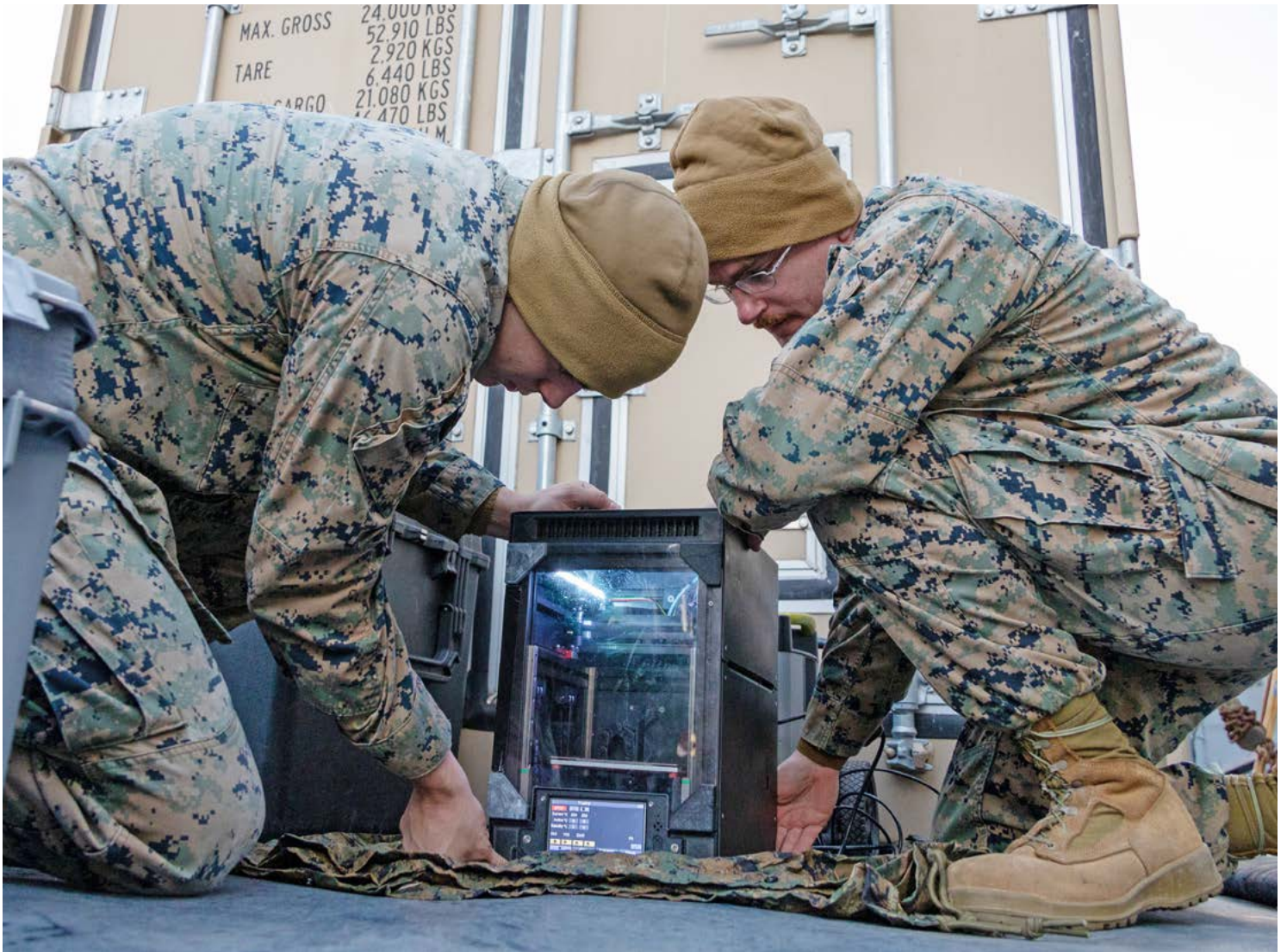
Marine Corps machinists with 1st Maintenance Battalion, 1st Marine Logistic Group assemble a 3D printer on Navy Landing Craft Utility 1665 in preparation to demonstrate expeditionary 3D printing capabilities. A recent CTMA project is working to streamline the advanced manufacturing hardware and software risk management process, to enhance manufacturing of replacement parts while in theater. (US Marine Corps photo by Sgt. Anabel Abreu Rodriguez.)
