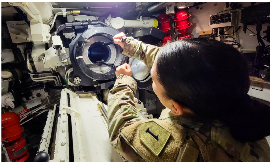
An armament repairer stationed at Pabrade Training Area, Lithuania, inspects the tracked vehicle barrel of a M109A7 Paladin. (US Army photo by 113th Mobile Public Affairs.)
