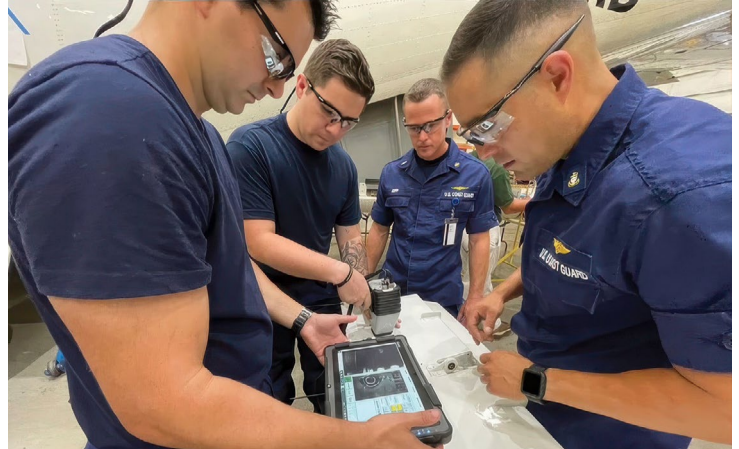
Technicians test out the Grey Gecko Real-Time Inspection Tool (GRIT) 125v2.5, a handheld, battery-powered system that uses spread-spectrum infrared technology. (Photo courtesy of Grey Gecko.)
