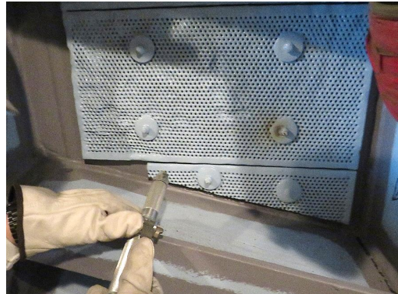
Figure 38: Sample Spot 18-3 (Center Left) Washer and Bolt Sound Tile Mount on Sub Mockup March 12, 2020
