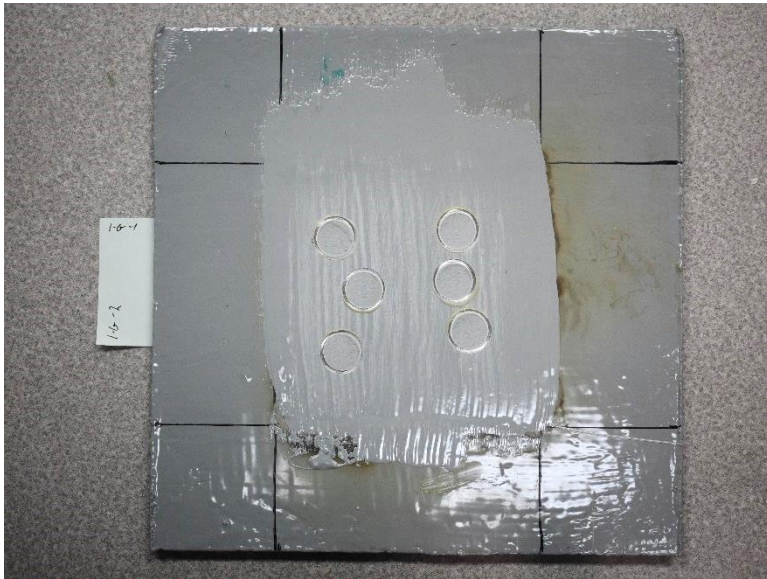
Figure 27: APCR Sample 1-G-1 After Dolly-Pull Coating Adhesion Testing
