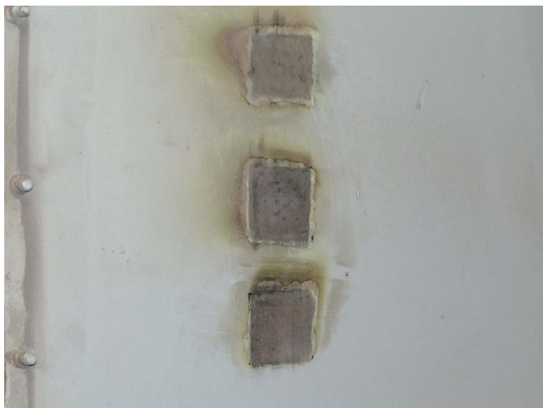
Figure 41: Sample Spots 17-1 After APCR Treatment March 12, 2020
