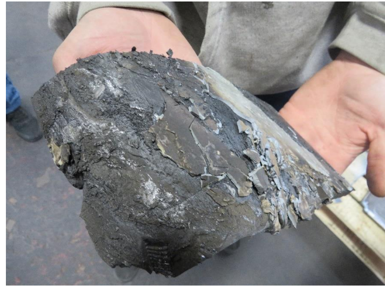
Figure 60: Sample Tile 3-R-7 After Removal Via APCR March 11, 2020
