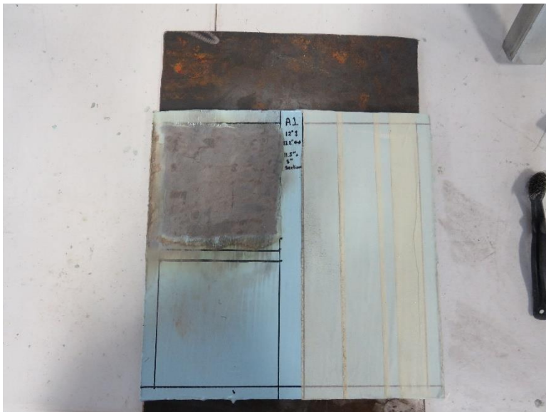
Figure 15: Sample A-1 After APCR Treatment August 27, 2020
