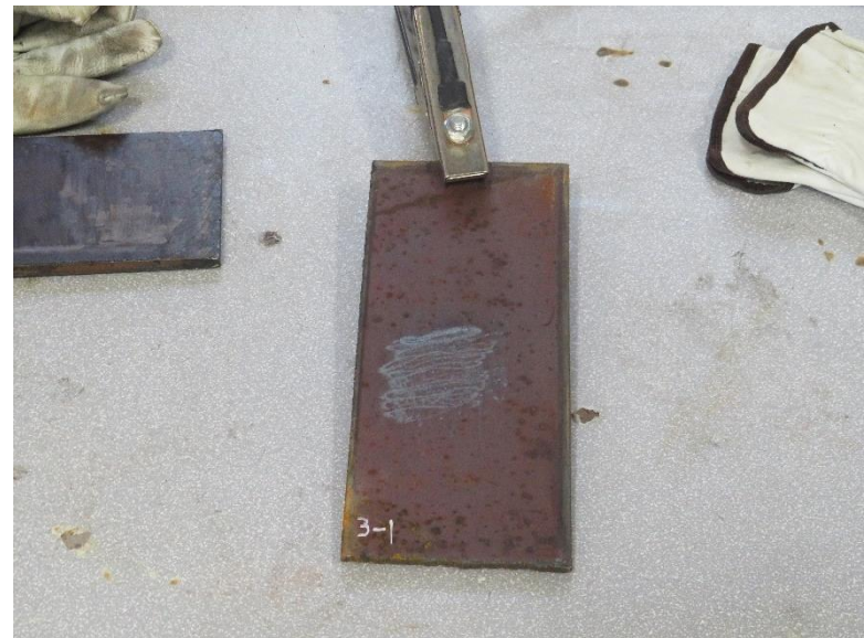
Figure 70: Salt-Contaminated Sample 3-1 After Plasma Treatment March 12, 2020
