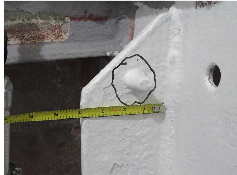
Figure 48: Sample Spot Sail-2-2 Welded Steel Bolt on Sub Sail Mockup March 13, 2020
