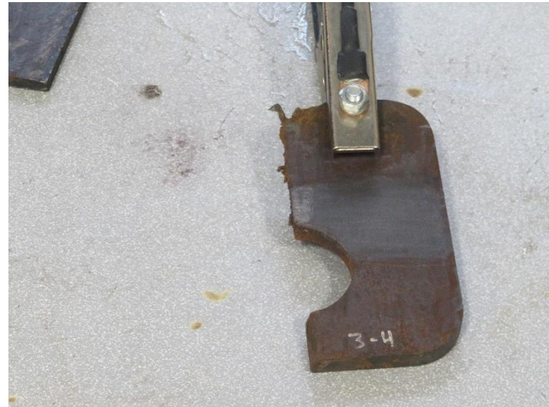
Figure 68: Salt-Contaminated Sample 3-4 After Second Plasma Treatment March 12, 2020
