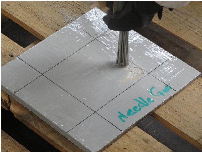
Figure 7: Flat Panel Sample Receiving Needle Gun Treatment March 12, 2020
