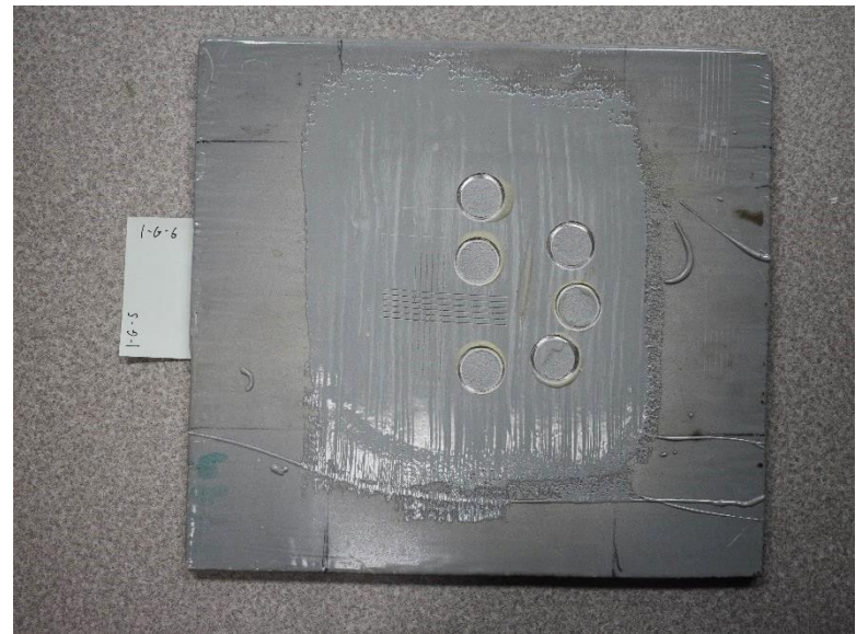
Figure 30: Abrasive Blasted Sample 1-G-6 After Dolly-Pull Coating Adhesion Testing
