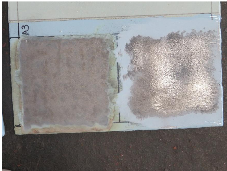
Figure 23: Sample A-3 After APCR (Left) and Needle Gun and Grinding (Right) August 27, 2020
