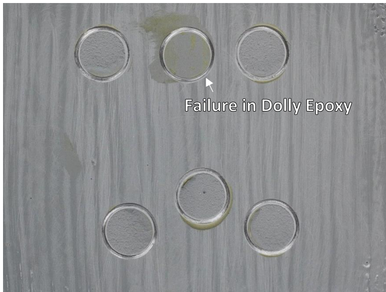
Figure 33: Abrasive Blasted Sample 1-G-5 Dolly-Pull Locations; One Failure Occurred in the Dolly Epoxy Adhesive
