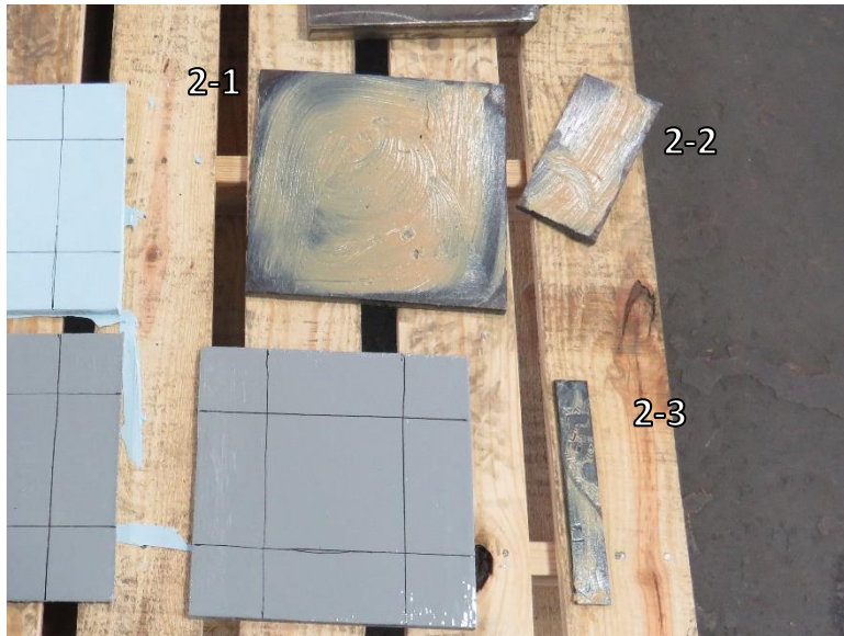
Figure 71: Grease Coated Samples 2-1, 2-2, 2-3 Before Treatment March 11, 2020
