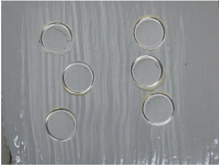
Figure 31: APCR Sample 1-G-1 Dolly-Pull Locations; All Failures were Cohesive Failures in the Body of the Coating
