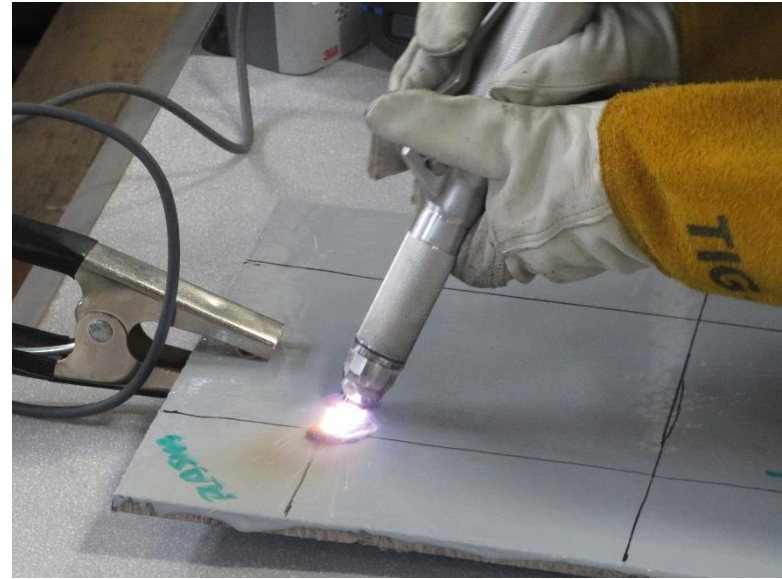
Figure 6: Flat Panel Sample Receiving APCR Treatment March 12, 2020
