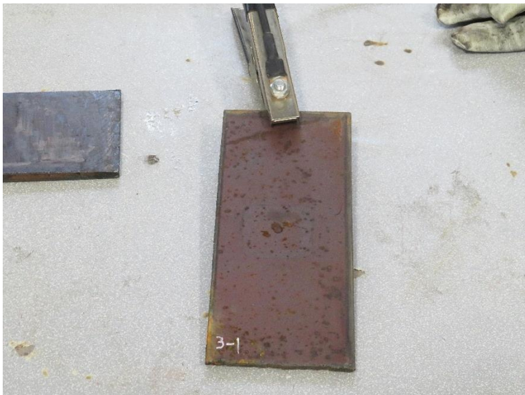
Figure 69: Salt-Contaminated Sample 3-1 After Bresle Patch Test, Before Plasma Treatment March 12, 2020
