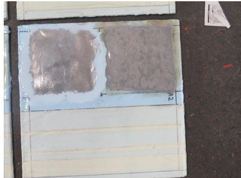
Figure 22: Sample A-2 After APCR (right) and Needle Gun and Grinding (Left) August 27, 2020
