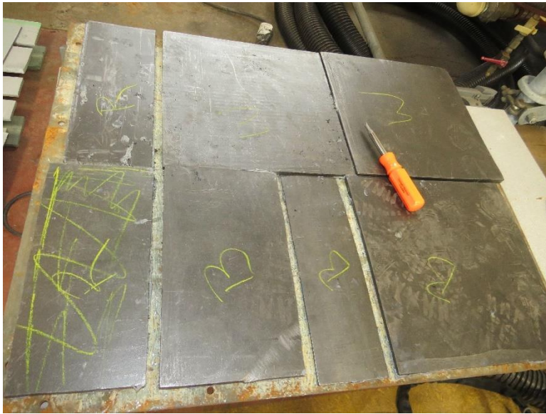
Figure 59: Rubber SHT Sound Tile Samples Prepared on Bare Steel Sheet March 11, 2020
