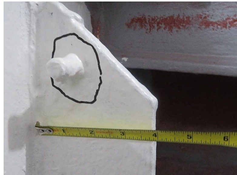
Figure 50: Sample Spot Sail-1-2 Welded Steel Bolt on Sub Sail Mockup March 13, 2020
