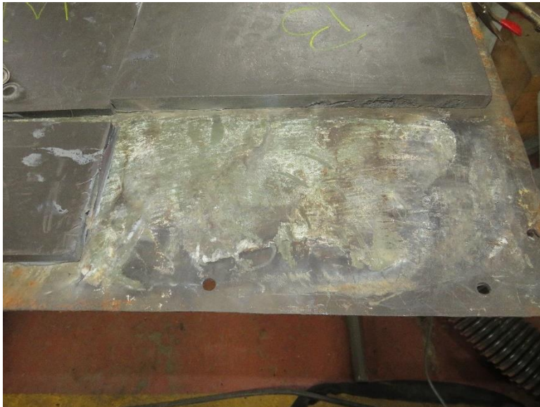
Figure 61: Steel Sheet Substrate After Removal of Sample 4-R-7 via APCR March 11, 2020
