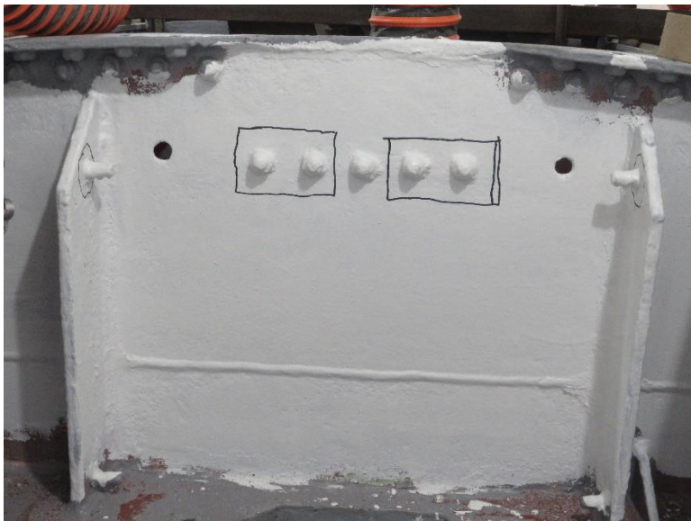
Figure 49: Sample Spots Sail-1 and Sail-2 Welded Nuts and Bolts on Sub Sail Mockup March 13, 2020
