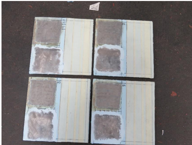
Figure 25: Samples A-1, A-2, A-3, A-4 After APCR and Needle Gun Treatments August 27, 2020
