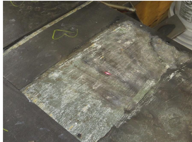
Figure 62: Steel Sheet Substrate After Removal of Sample 4-B-5 via APCR March 11, 2020
