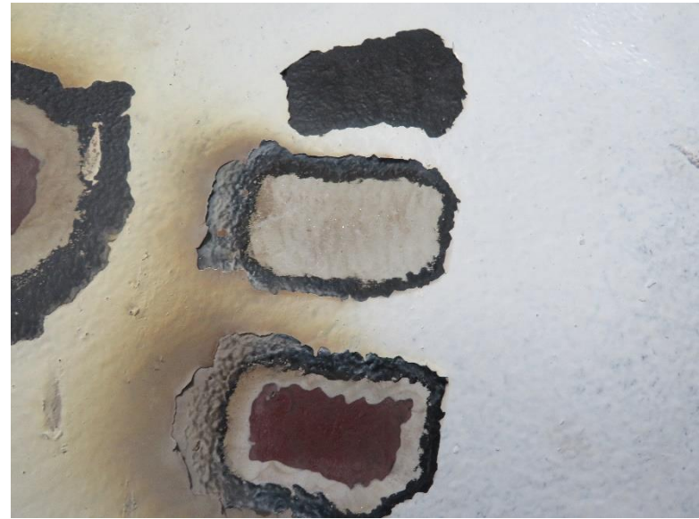
Figure 76: Demonstration of Selective Layer Removal with PlasmaBlast ® Tool March 13, 2020
