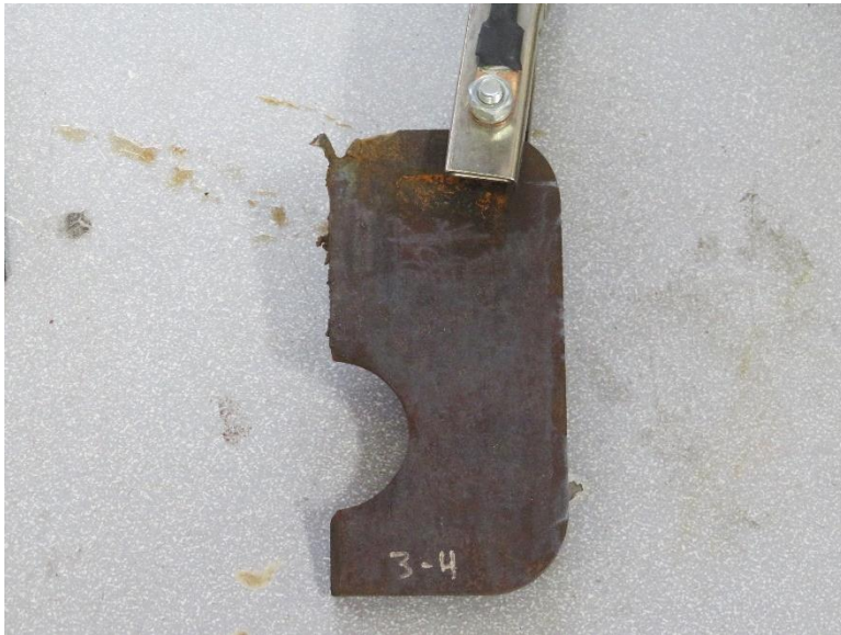
Figure 67: Salt Contaminated Sample 3-4 After First Plasma Treatment March 12, 2020
