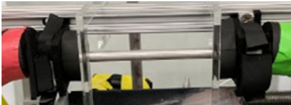
Figure 10. Close-Up of Coated Tube in Test Apparatus
