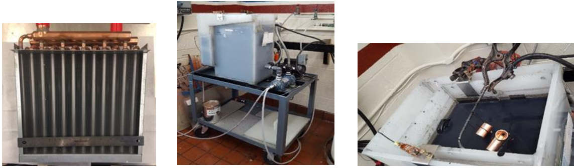
Figure 25. Uncoated Heat Exchanger (left); Custom Built 11-Gallon Bath (center): Top Down View of Bath Filled with Electrodeposition Coating (right)
