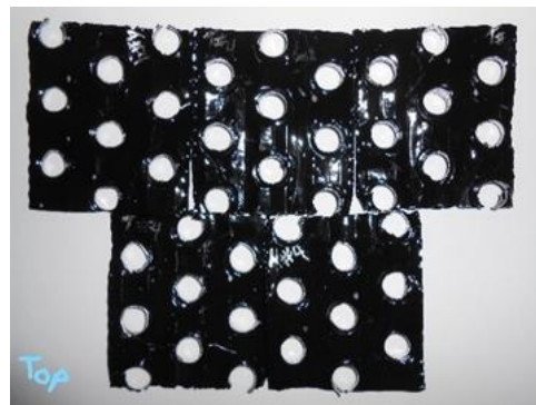
Figure 24. Electrocoated Heat Exchanger Fins After Coating and Disassembly
