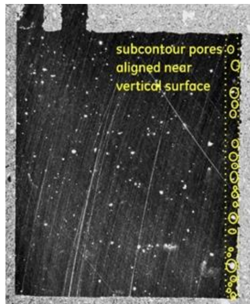
Figure 5. Illustration of Sub-Contour Porosity in Low Sa Sample from DOE3a Sub-contour pores are circled in yellow
