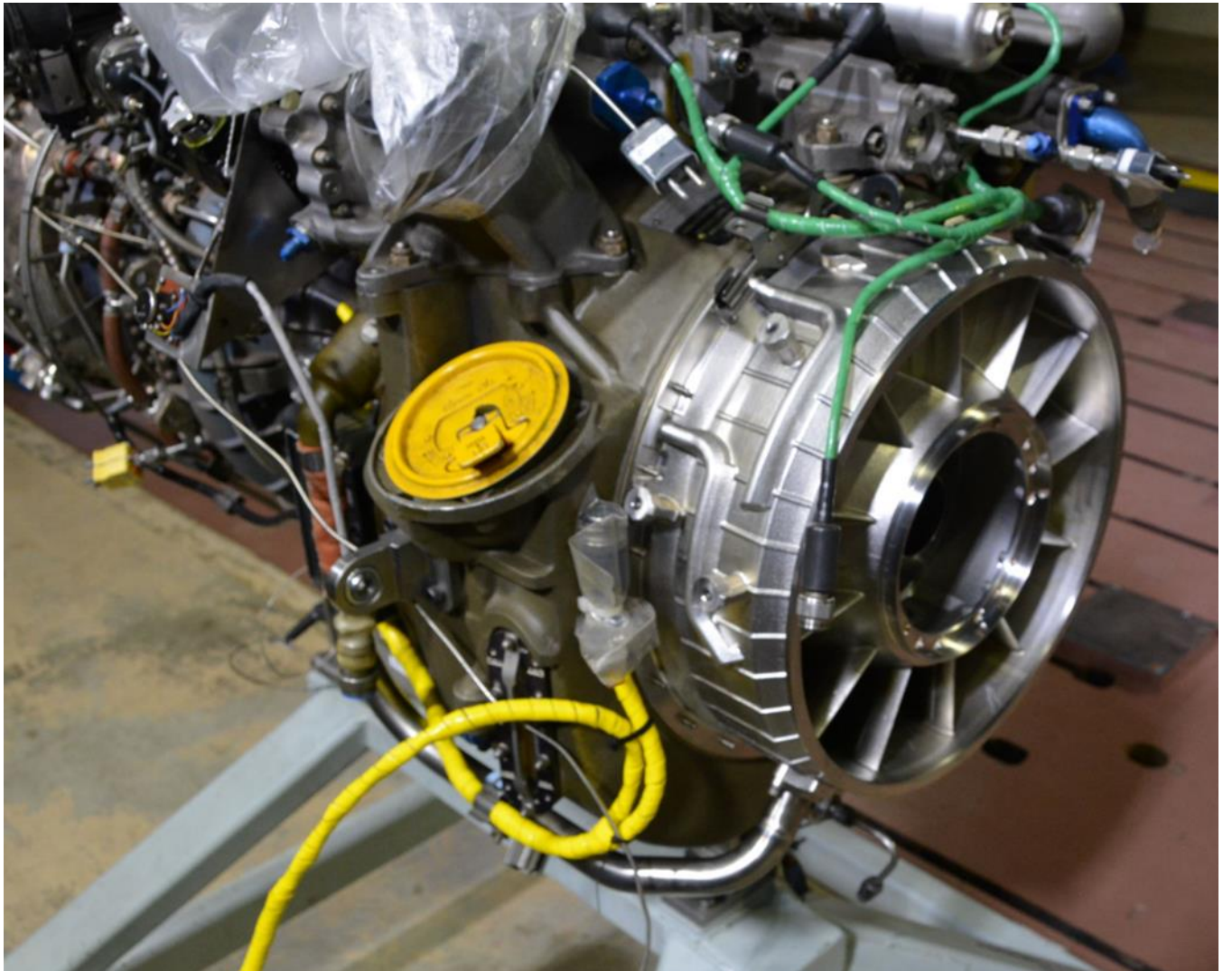
Figure 58. Final Assembly Fit Check – 17A206-230G01 Additive Swirl Frame Installed on U.S. Navy T700-401C Engine Photo courtesy of Naval Air Systems Command (NAVAIR)
