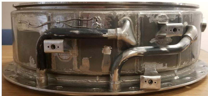
Figure 51. Flight Counter Mounting Brackets on Production Swirl Frame (6053T29)
