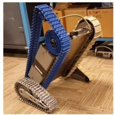
Figure 3-18. Hand Stand and Rotation Tested per CCDC-GVSC Repair Protocol
