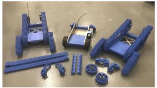
Figure 4-9. Three Configurable GVR-BOTs Showcasing AM Potential
