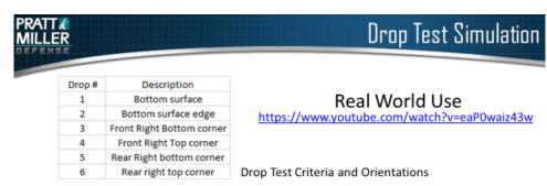
"The test item (the robot and the OCU each) will be subjected to Handling Drop Shock IAW MIL-STD-810F Method 515.5, paragraph 4.5.5.1 and Table 516.5-VI.
