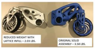
Figure 4-6. Caster Arm Design With and Without Lattice Optimization
