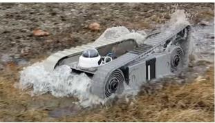
Figure 3-16. Forging Test and First Test of the Track and Tensioner System
