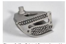
Figure 5-17. Printed Caster Arm with Lattice Filled Interior
