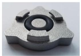
Figure 3-13. Tapered Tab and O-Ring Sealing Test
