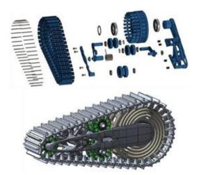
Figure 4-4. Complex Assembly with Multiple Bearings and Springs Done Without Any Secondary Machining
