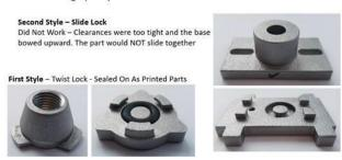
Figure 4-2. Sealing and Tapered Post Feature Test Parts
