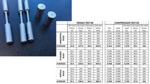
Figure 3-8. Material and Process Test Coupons and Results
