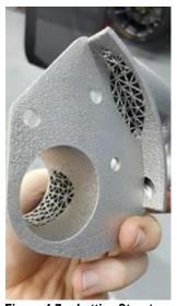
Figure 4-7. Lattice Structure in Caster Arm
