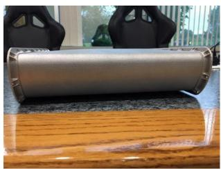
Figure 4-11. Distorted Housing with No Ribs or Corrugation
