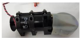
Figure 3-5. Original Motor and Gearbox with Grease Cover
