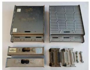
Figure 3-3. Direct Replacement of Parts from Scan Data and Material Analysis
