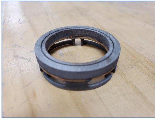
Figure 94. AGB Rotor After Welding, Prior to Machining
