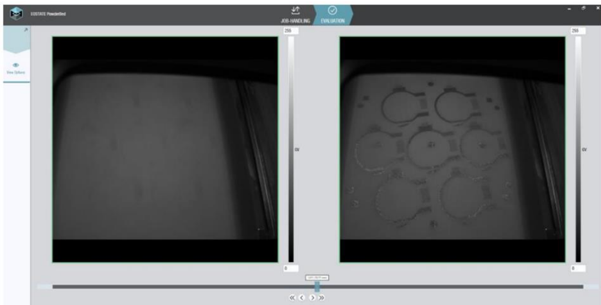
Figure 102. EOSTATE Powder Bed Images
