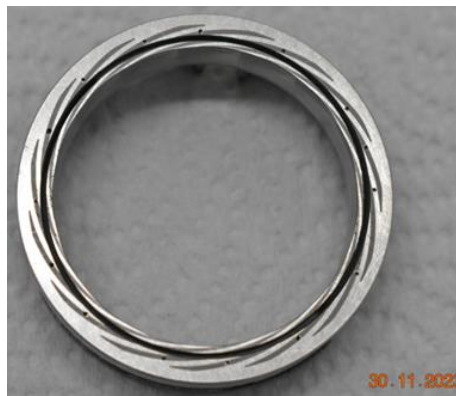
Figure 95. AM Mating Ring with Hydrodynamic Pads and Holes in Face
