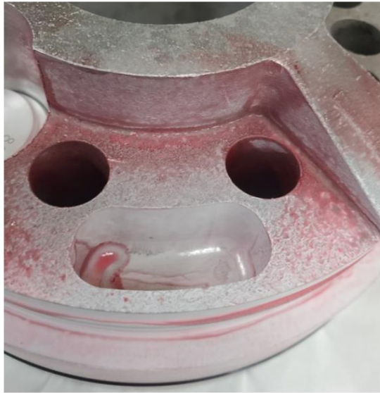
Figure 65. Typical Intermediate FPI of AM AISi10Mg Port and Pressure Plate Component
