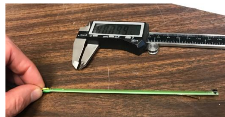
Figure 2. Probe Disassembled with 0.125" Sensor to the Right Used to test functionality of the probe in restricted geometry such as inside features in the tube
