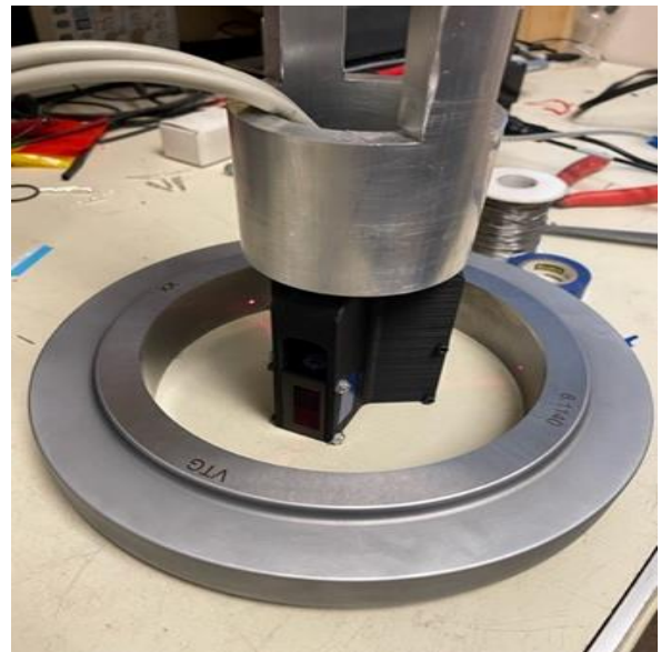
Figure 11. Triangulation Sensors Bench Top Testing in Gauge Ring
