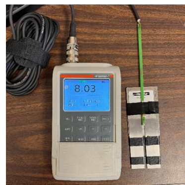
Figure 3. Testing of Sensor in Feature Mock-Up Showed Interference of Sidewalls Leading to Inconsistent Results
