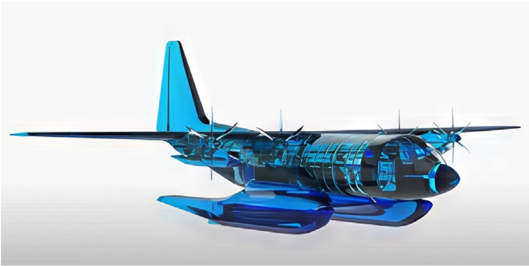
This rendering depicts an MC-130J with a removable amphibious float modification for which a CTMA project initiated development, resulting in the fabrication of a kit for operational demo. (USAF digital illustration.)
