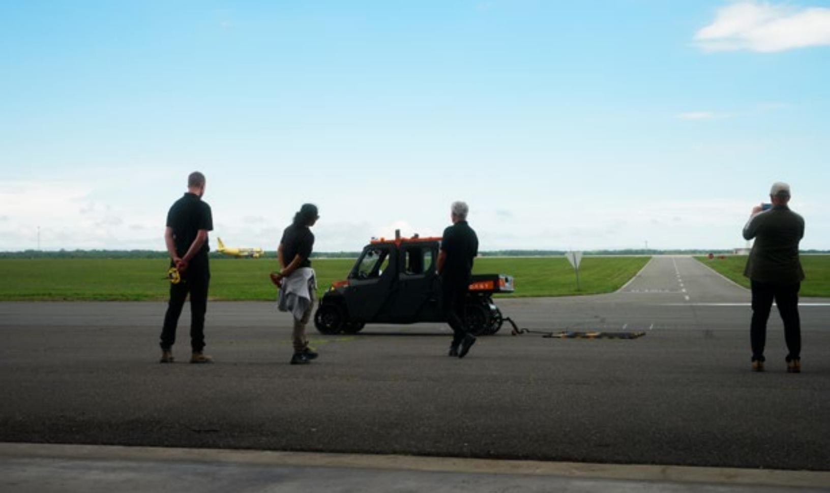
COAST Autonomous demonstrated their foreign object debris (FOD) Pro XD Autonomous Road Machine (ARM), based on a modified Polaris Pro XD utility task vehicle, equipped with a FOD*BOSS sweeper. (Photo by Travis Shea.)
