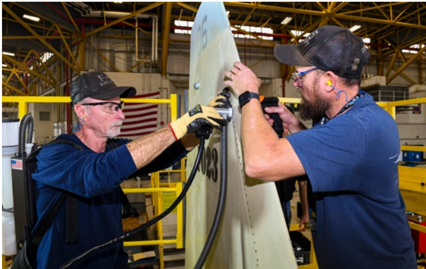
The Fleet Readiness Center Southeast F-5 Aircraft Production Line uses the E-Drill system to remove metal fasteners on an F-5 Tiger II vertical stabilizer. (US Navy Photo by Toiette Jackson.)
