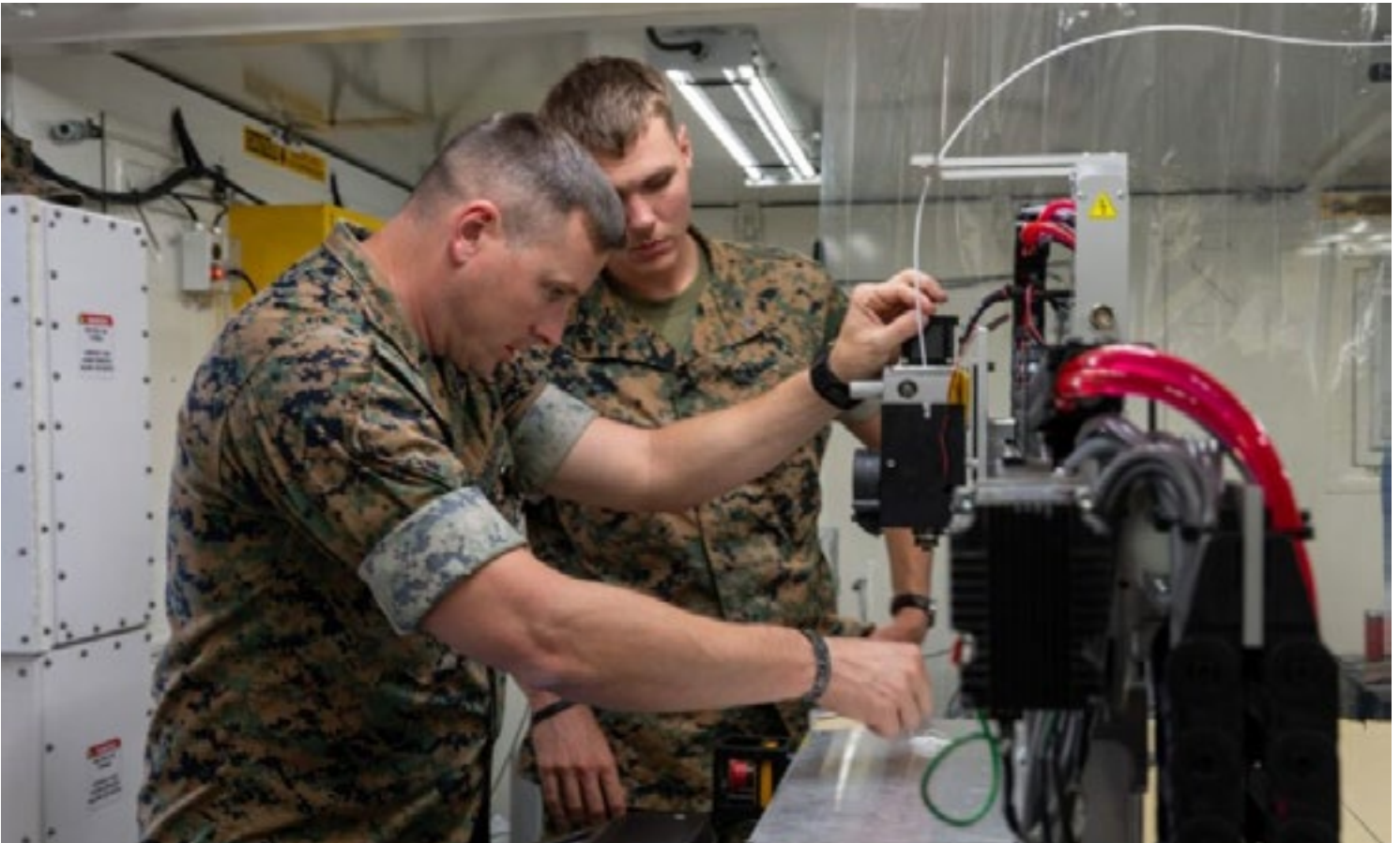
US Marines test out an expeditionary fabrication lab developed in 2023, equipped with multiple 3D printers, scanners, laser cutters and other support tools. Its design informed the recent CTMA project team that developed a new portable AM lab. (U.S. Navy photo by Michael Walls.)
