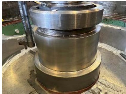
On-Board Rudder Stock Repair
