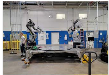
World's largest high throughput large scale cold spray AM cell
