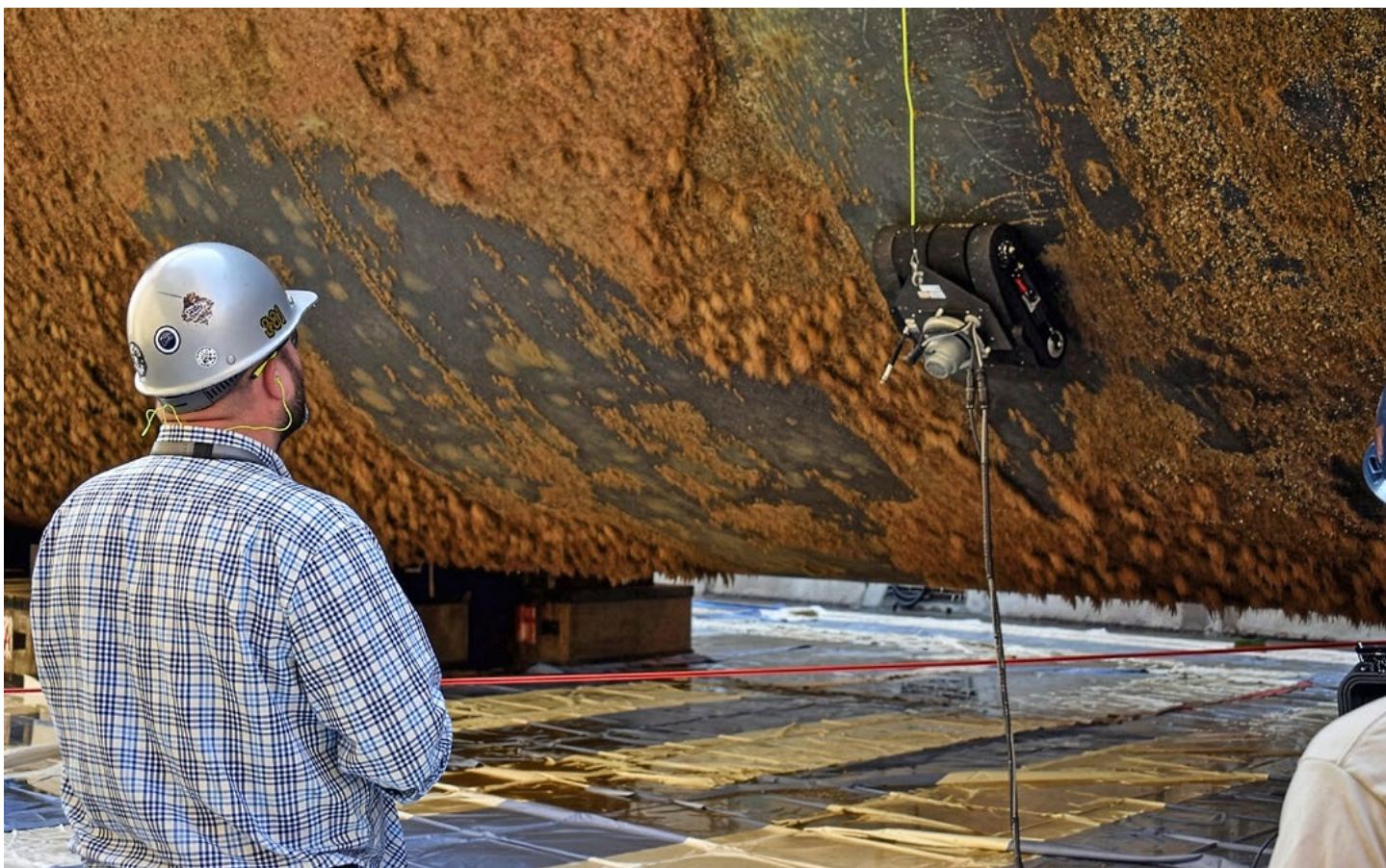
An operator demonstrates the vacuum crawler robotic system that has been ruggedized by Boston Engineering for removing biofouling from Navy vessels. (Photo courtesy of Boston Engineering.)
