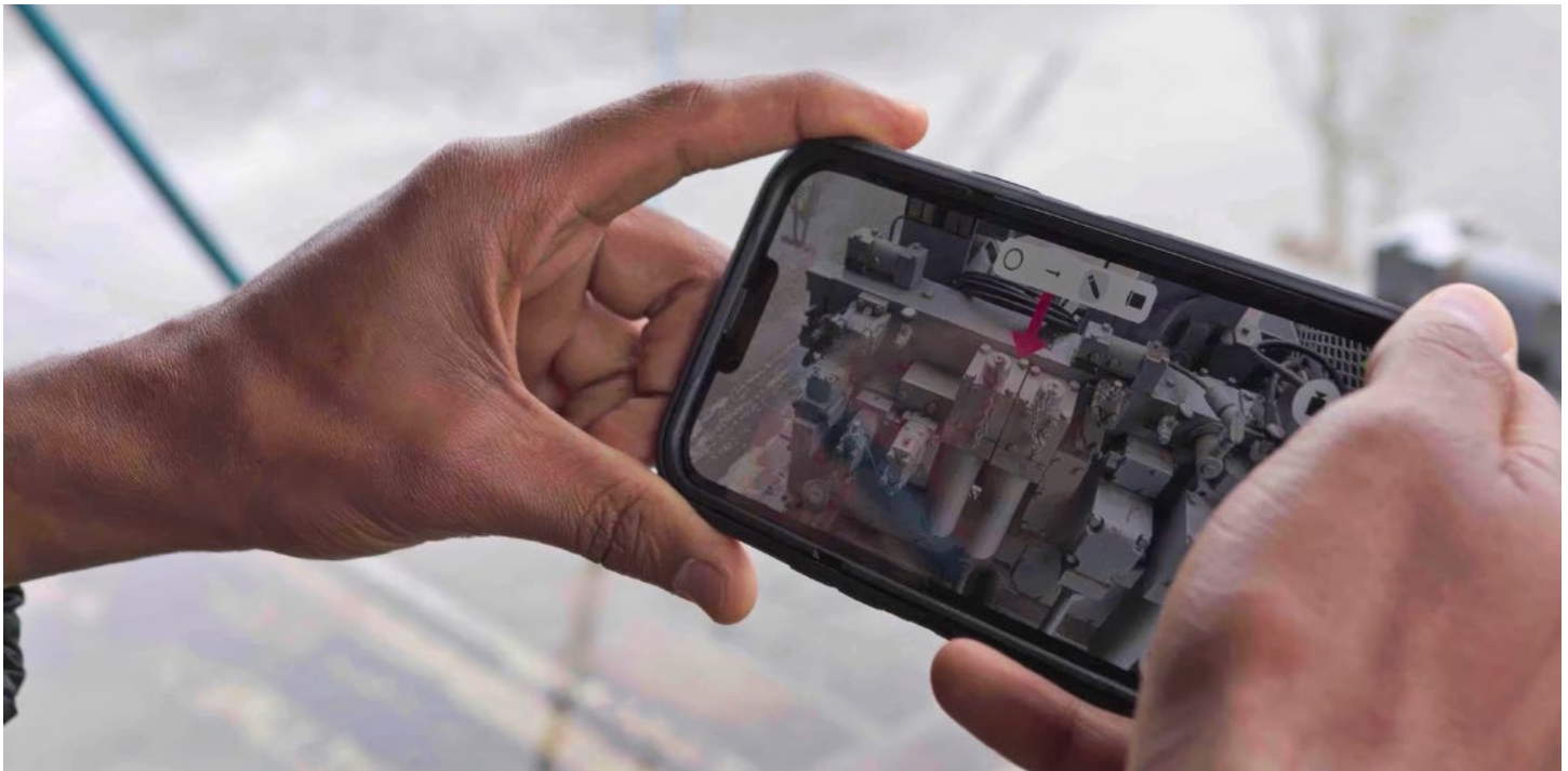
The Mixed Reality Expert Guidance (MREG) system is a remote assistance platform produced by Boston Engineering that enables technicians in the field to contact subject matter experts via a secure, remote connection to seek guidance with real-time audio and video supplemented by AR-enhanced visual aids. (Still image captured from US Navy video by Eric M. Osborne and Marco Hinahon.)
