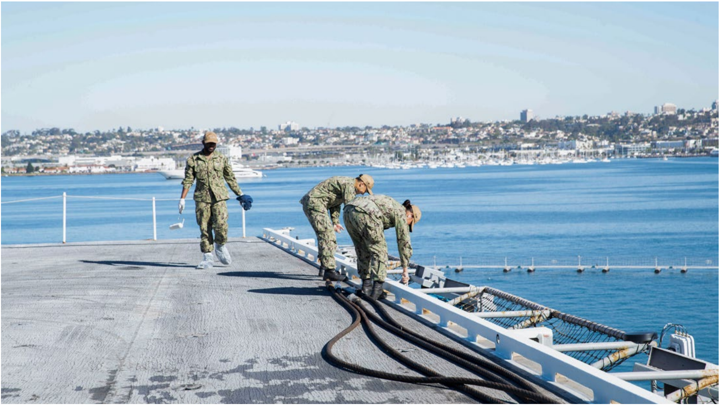
Sailors paint scuppers—one method used to prevent corrosion—on the flight deck of the Nimitz-class aircraft carrier USS Abraham Lincoln while moored at Naval Air Station North Island in San Diego, CA. (US Navy photo by Mass Communication Specialist Seaman Apprentice Melanie Perez.)
