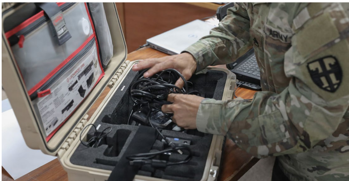
A technician from the Puerto Rico Army National Guard prepares a maintenance support device used to gather maintenance data for ground vehicles in real time. (US Army National Guard photo by Spc. Deneiz Agosto Camacho.)
